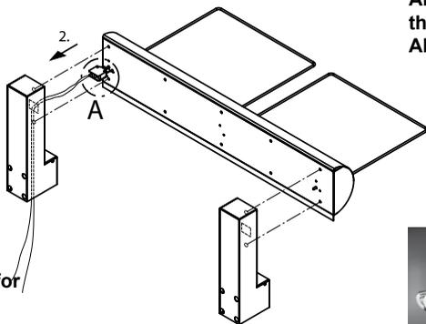
Lay the control cable for the rocker switch and heater supply with a minimum clearance of 30 mm.
